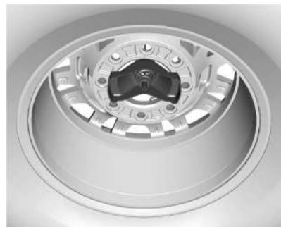
ZR2 Model Correctly Stored, Retainer Centered
