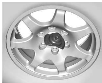
All Other Models Incorrectly Stored, Retainer Off-Center
