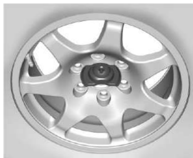
All Other Models Correctly Stored, Retainer Centered
