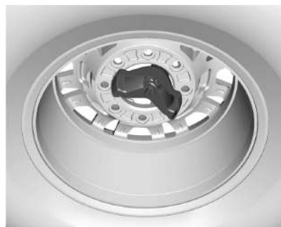
ZR2 Model Incorrectly Stored, Retainer Off-Center
