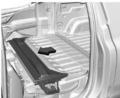
Midgate Lowered with Crossbar Attached
