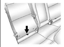
Flip the seat cushion forward by pulling up on the tab in the center of the seat cushion where the seatback meets the seat bottom.
