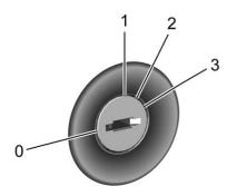
The ignition switch has four different positions.
