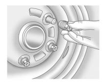
Reinstall the wheel nuts with the rounded end of the nuts toward the wheel. Tighten each nut clockwise by hand until the wheel is held against the hub.
