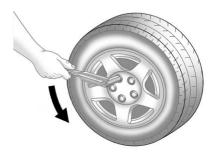
To remove the plastic covers and wheel nut caps, loosen the plastic nut caps with the wheel wrench in a counterclockwise direction.
