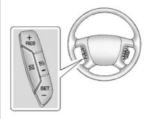
(c) (On/Off): Press to turn cruise control on or off. A white indicator comes on in the instrument cluster when cruise is on.
