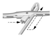
Lift up on the plastic latch in the middle of the wiper blade where the wiper arm attaches.
