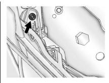
13. Reinstall the screw from the headlamp assembly.
