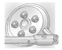
Turn the wheel wrench counterclockwise once on each wheel nut to loosen it. Do not remove them yet.
