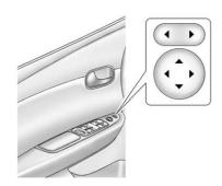
Controls for the outside power mirrors are located on the driver door armrest.
