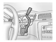
**P**: This position locks the front wheels. It is the best position to use when starting the engine because the vehicle cannot move easily.
