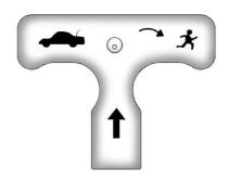
There is a glow-in-the-dark trunk release handle located on the latch inside the trunk. This handle will glow following exposure to light. Pull the release handle to open the trunk from the inside.
