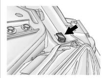
12. Push down on the plastic headlamp retainer to reinstall it.
