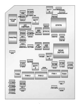
The vehicle may not have all of the fuses, relays, and features shown.
