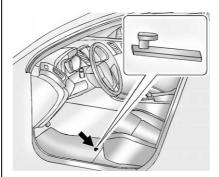
The driver side floor mat is held in place by one hook-type retainer.
