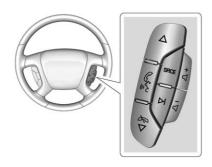
If equipped, these controls are located on the right side of the steering wheel.
