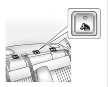
The top tether anchors are under the covers on the rear seatback filler panel. Be sure to use an anchor on the same side of the vehicle as the seating position where the child restraint will be placed.
