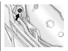
Remove the screw from the headlamp assembly.
