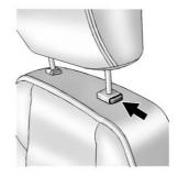
To lower the head restraint, press the button located on top of the seatback, and push the head restraint down. Try to move the head restraint after the button is released to make sure that it is locked in place.
