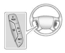
(S): Press to turn cruise control on or off. A white indicator comes on in the instrument cluster when cruise is on.
