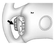
ERS mode allows you to choose the top-gear limit of the transmission, which can help control the vehicle's speed while driving downhill or towing a trailer. The vehicle has an electronic shift position indicator within the instrument cluster. When using the ERS mode a number will display next to the L, indicating the current range that has been selected.
