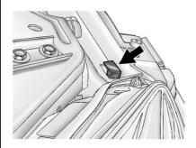
3. Pull up on the plastic headlamp retainer and remove it.
