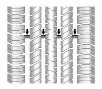
Treadwear indicators are one way to tell when it is time for new tires. Treadwear indicators appear when the tires have only 1.6 mm (1/16 in) or less of tread remaining. See *Tire Inspection* ⇒ 240 and *Tire Rotation* ⇒ 240.
