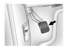
The parking brake is located to the left of the brake pedal, near the driver door.
