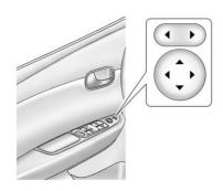
Controls for the outside power mirrors are on the driver door armrest.
