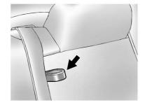
Lower the seatback by pulling forward on the tab on the outboard side of the rear seatback.
