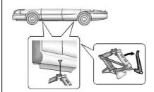
3. For all wheel types, find the jacking location using the diagram above and the corresponding jacking notches located on the bottom side of the plastic molding. The notches in the plastic molding are marked with a triangle shape to help you find them.
