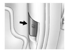
The fuse block is on the passenger side of the vehicle in the carpet molding. Remove the fuse block door to access the fuses.
