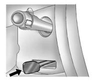
The tilt wheel lever is located on the left side of the steering column.
